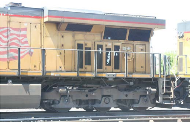
A nice detail shot of the radiator and dynamic brake section of an ES44.
